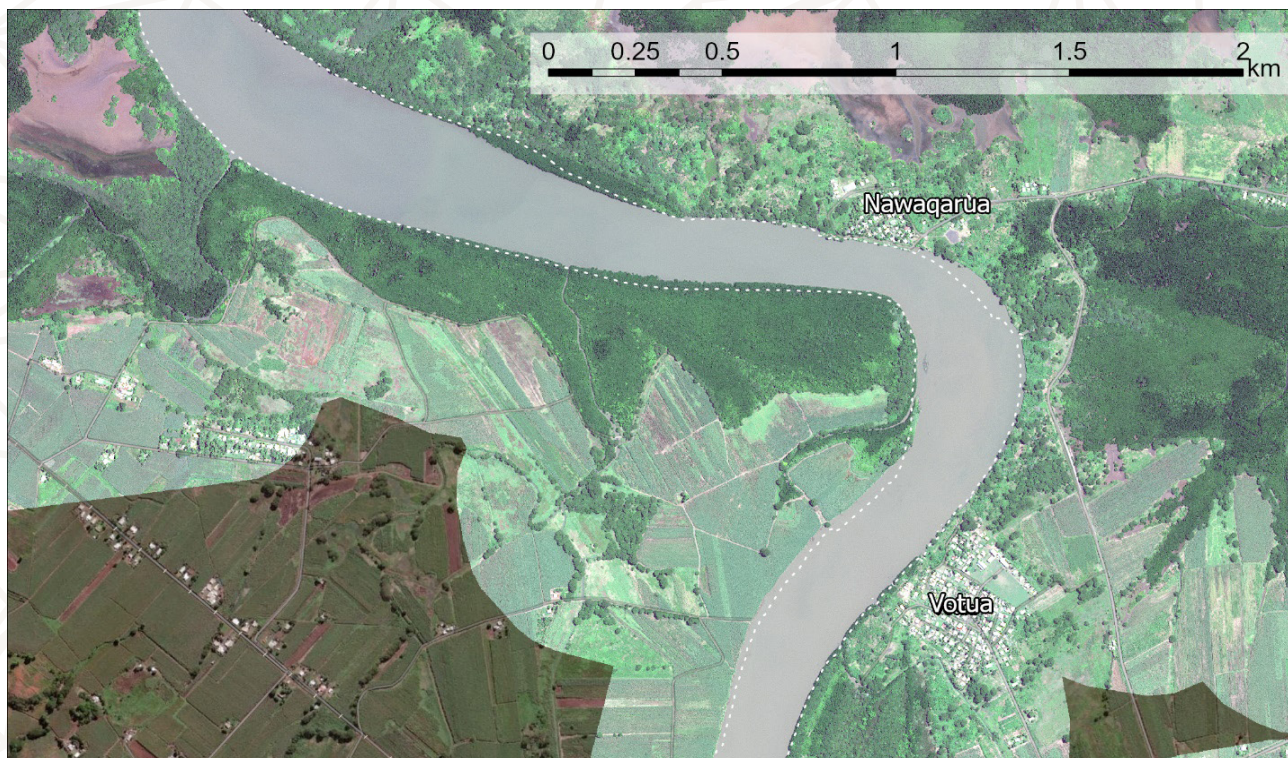
Figure 13. Erosion and accretion along the riverbank resulting in change in mangrove extent near the villages of Nawaqarua and Votua in Ba Delta. The satellite image shows the margin of the river in April 2022, and the white dotted line shows the margin of the river delineated based on satellite imagery from August 2010.
